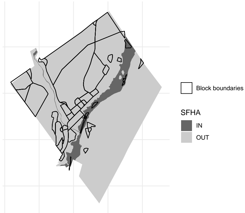
Figure C.6: Census Blocks and the SFHA Zones for Village of Delhi, NY (8% SFHA)
